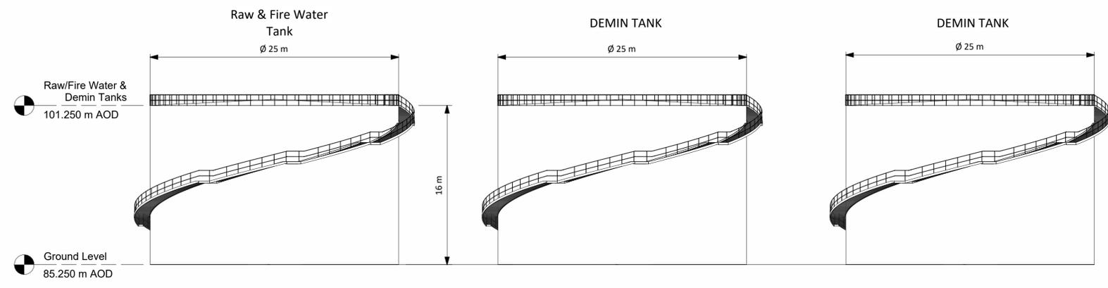
**3 Fire/Raw Water & Demin Tank West Elevation**
