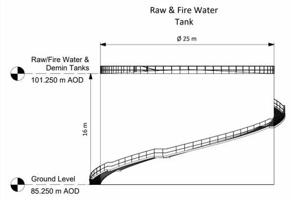
**2 Fire/Raw Water & Demin Tank North Elevation**
