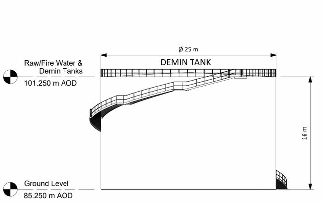
**4 Fire/Raw Water & Demin Tank South Elevation**
