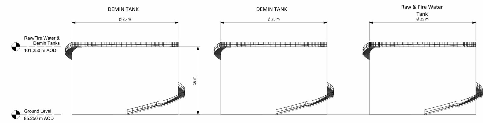
**5 Fire/Raw Water & Demin Tank East Elevation**
